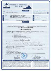
Galvanized Steel Accelerated Corrosion Test
